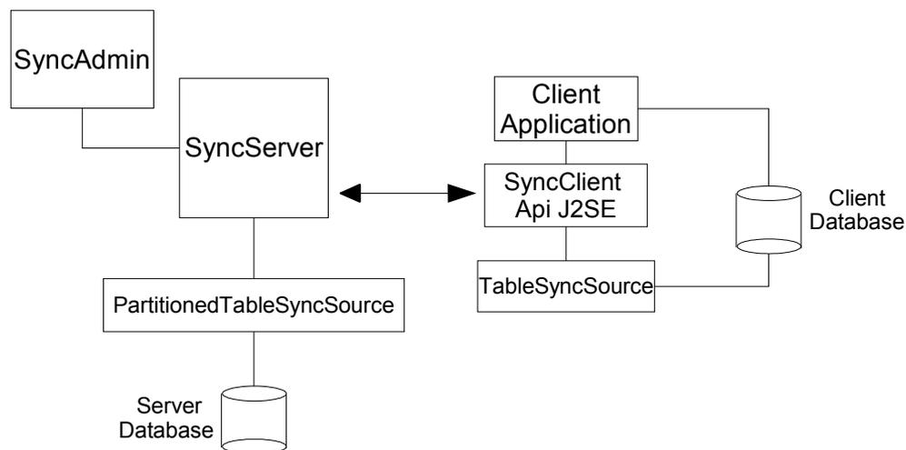
*Figure 11 - Sync4j DB Connector high level architecture*
