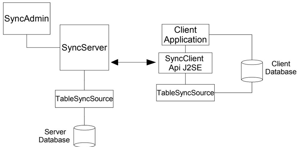
Figure 6 - Sync4j DB Connector high level architecture
